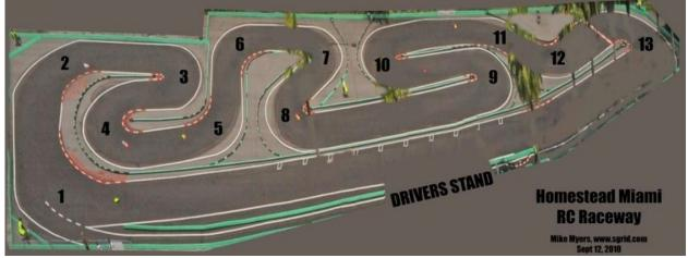
Track length: 960 feet / 292.6 meters Track width: 15-18 feet / 4.57-5.48 meters Pit lane width: 5 feet / 1.52 meters Straightaway width: 15-18 feet / 4.57-5.48 meters Straightaway length: 275 feet / 83.82 meters Driving direction: Clockwise
